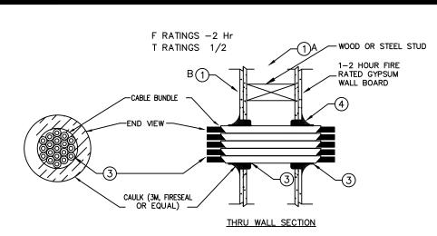
1. WALL ASSEMBLY – THE FIRE-RATED GYPSUM WALLBOARD/STUD WALL ASSEMBLY SHALL BE CONSTRUCTED OF THE MATERIALS AND IN THE MANNER DESCRIBED IN THE INDIVIDUAL U300 OR U400 OF SERIES WALL OR PARTITION DESIGNS IN THE UL FIRE RESISTANCE DIRECTORY AND SHALL INCLUDE THE FOLLOWING CONSTRUCTION FEATURES: A. STUDS - WALL FRAMING MAY CONSIST OF EITHER WOOD STUDS (MAX 2H FIRE RATED
